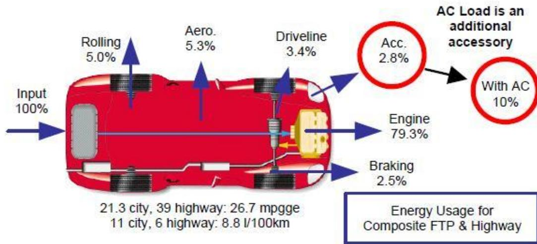
Figure 4 - Energy Usage for an Average 27 mpg Vehicle [4]
