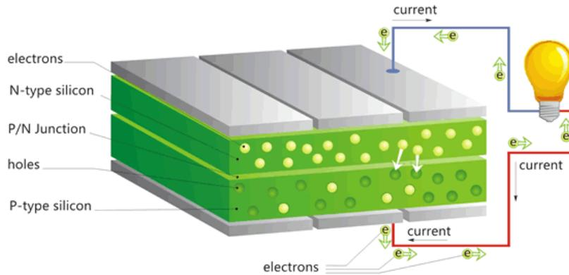
**Figure 2 - Solar Cell Circuit [2]**
