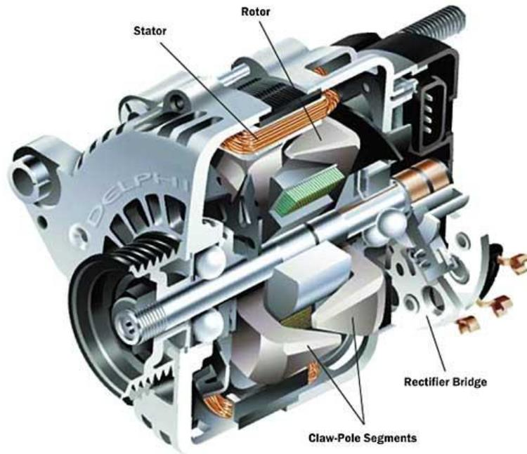
**Figure 9 - Automotive Alternator [9]**
