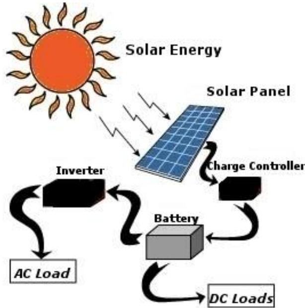
Figure 3 - Typical Solar Energy System [3]
