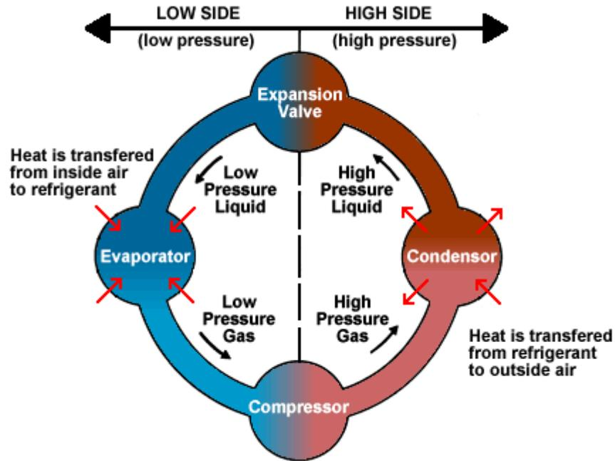
Figure 8 - Air Conditioning Cycle [8]
