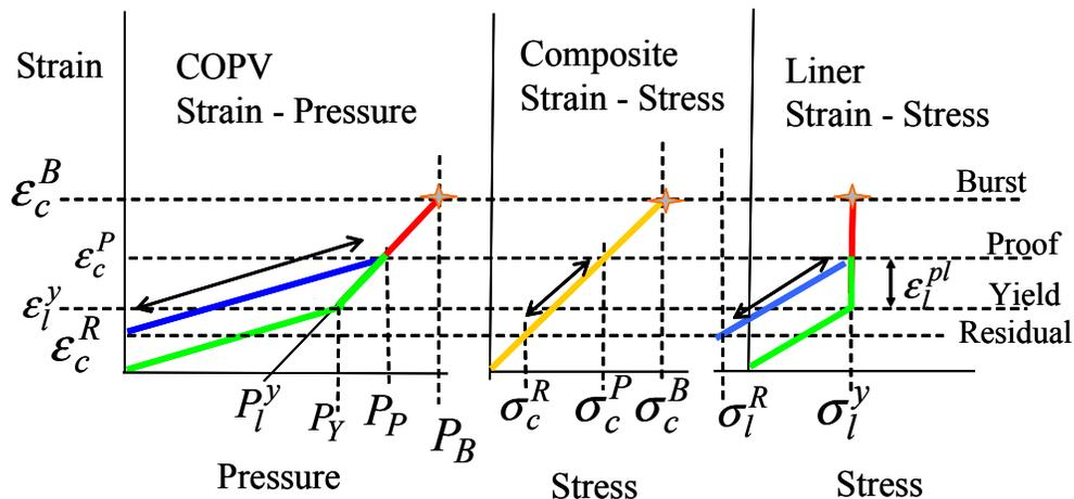
Figure 2. Strain– pressure/stress relationships based on continuity of strain for COPV vessel, composite and liner respectively. Operational loads from  $P=0$  to MEOP lie on the blue line for pressures less than  $P_P$
