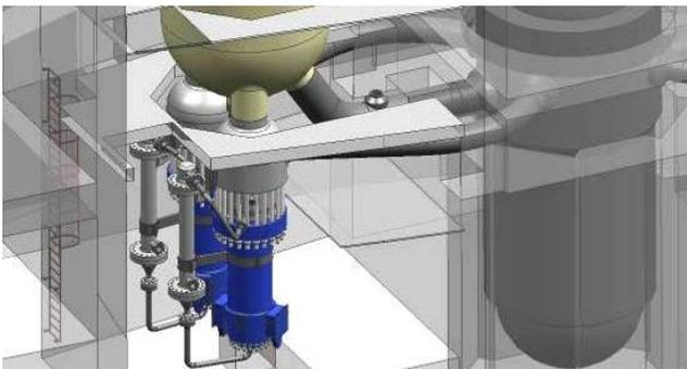
Fig. 1: Mounting position of the AP 1000 RCPs
