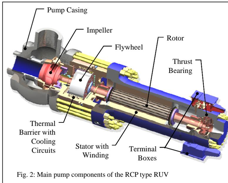
Fig. 2: Main pump components of the RCP type RUV
