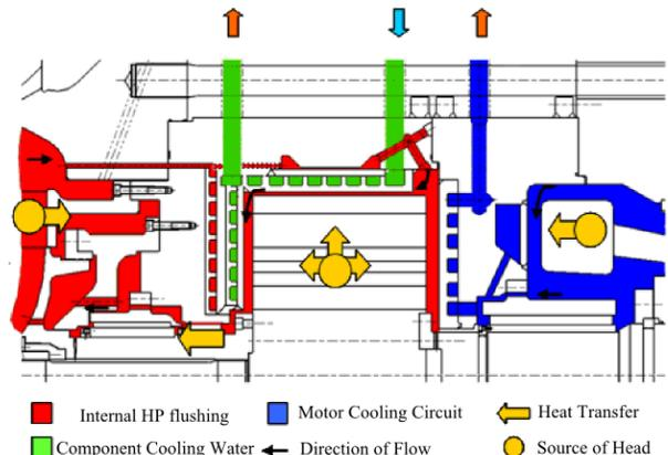
Fig. 5: Cooling circuits and heat transfer around the flywheel and within the heat barrier
