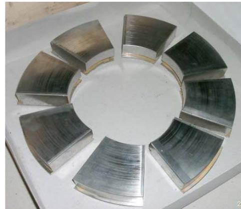
Fig. 14: Thrust bearing pads (stationary) after 6483 startup cycles.
