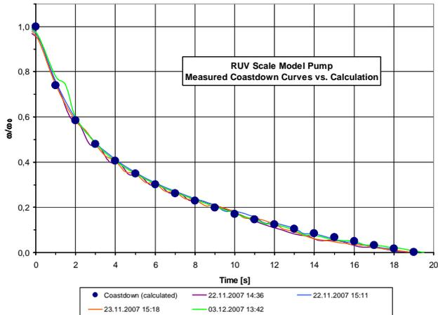
Fig. 12: Measured coastdowns curves vs. calculation
