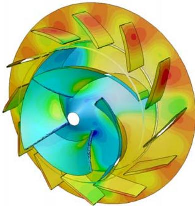
Fig. 11: CFD analysis of impeller/diffuser
