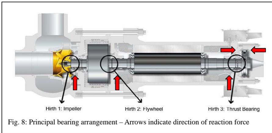
Fig. 8: Principal bearing arrangement – Arrows indicate direction of reaction force
