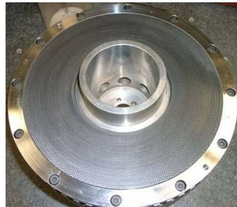
Fig. 13: Thrust bearing plate (rotating) after 6483 startup cycles.
