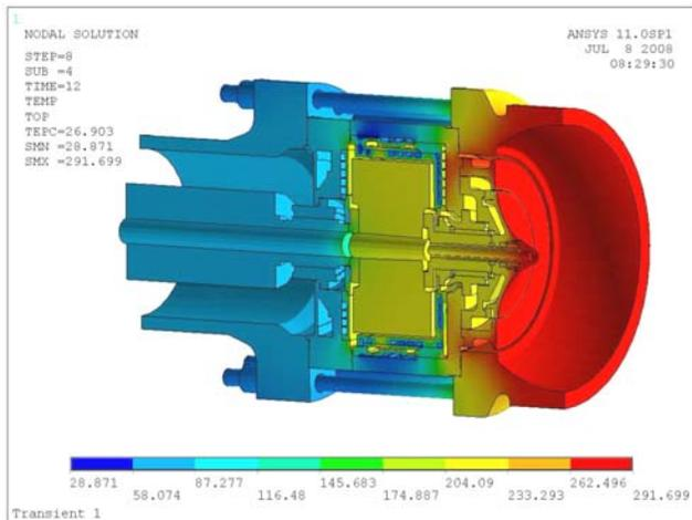
Fig. 4: Plot of the calculated temperature distribution in the heat barrier and surrounding areas (normal operation, steady state). Temperature unit is °C.
