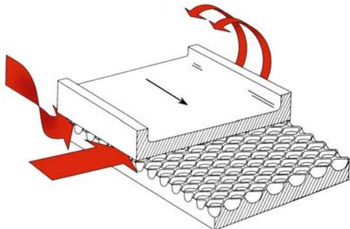
Fig. 9: Image of a cellular wear ring and its mode of action
