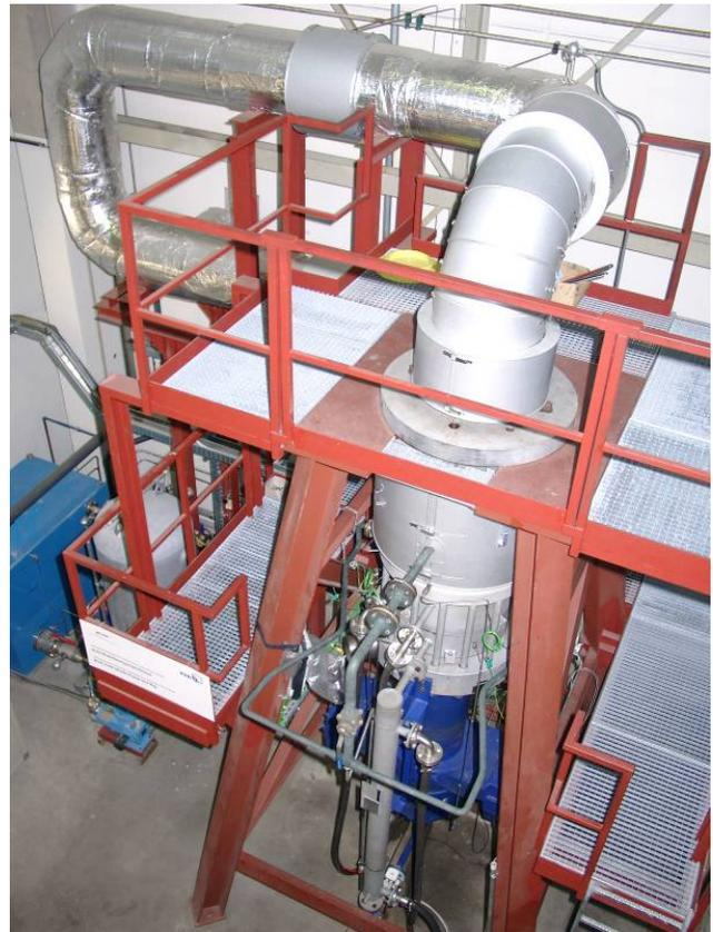
Fig. 10: Scale model pump with test rig
