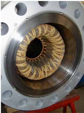
Fig. 6: View of a wet winding motor
