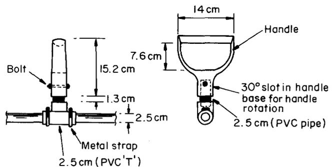
Figure 3 Detailed design of the secondary shaft of the modified shovel (dimensions in centimetres)
